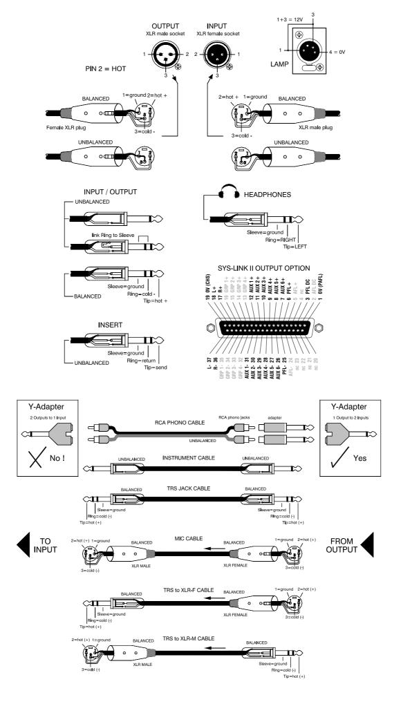
The MixWizard uses professional grade 3 pin XLR, 1/4" TRS (3 pole) jack and RCA phono sockets. To ensure best performance, we recommend that you use high quality audio cables and connectors, and take time to check for reliable and accurate cable assembly. It is well known that most audio system problems are due to faulty or sub standard interconnecting leads. The following plugs may be used to connect audio to the console:
