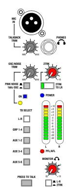
**TALKBACK** Individually assignable talkback is available to all the main outputs. Plug in a suitable cable or gooseneck microphone. A good quality dynamic or condenser vocal microphone is recommended. Note that +48V phantom power is available at the XLR as standard. If you prefer, this can be disabled by repositioning an internal jumper link.
