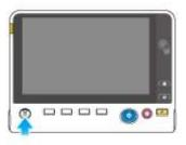
The **Power** key can be used as a power save key to manually switch to Power Save mode. Power Save mode is classified into two modes: Low Power mode and Sleep mode.
