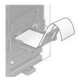
4. Slide the Lateral Guide to fit the size of the loaded paper.
