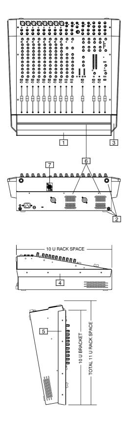
**Carry Handle** Metal handle for lifting and carrying the console. The weight is centrally distributed. Lift the console by holding the handle securely in the middle. To prevent damage to the controls, carry it with the control surface away from you.
