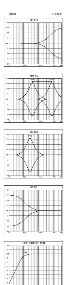
**EQUALISER** The channel equaliser allows independent adjustment of four frequency bands. This lets you accurately pinpoint the frequencies you want to adjust to deal with problems such as feedback or instrument resonance, or to creatively tailor the sound.
