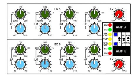
**Overview** The two built-in power amplifiers are called Amp A and Amp B. You decide how you want to use them. Different combinations of the LR, FB1 and FB2 mixes can be selected according to your preferred system setup. Each channel includes a 4-band semi-parametric equaliser for precise speaker/room frequency shaping. The level controls let you match the console signals to the speaker volume you require. A row of LED indicators display important information about the amplifier status.
