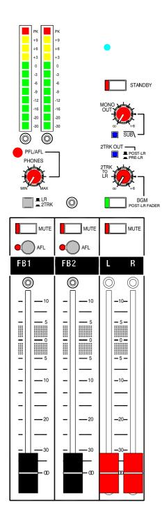
**Master Control** For accurate control, the main house and two foldback mixes are controlled using full length faders and include mute and headphone monitoring functions. These faders act as volume controls for the mix.
