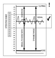
sound peaks. You need to consider the matching between the microphones and the (gain), channels inserted equipment (operating level and trims), channels to the mix (faders), and outputs into the amplifiers (level trims). The diagram here illustrates the principles of signal dynamics.
