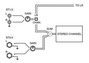
**Dual Stereo Inputs** Each stereo channel has two independent stereo inputs, ST1(3) and ST2(4). For convenience, one uses RCA phono connectors, the other uses TRS jacks. The two inputs mix together to feed the channel strip, or ST1(3) can be routed direct to the LR mix instead, leaving ST2(4) to feed the channel. This provides a very flexible arrangement for mixing up to four stereo sources.
