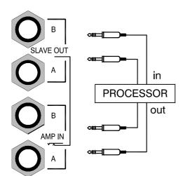
**AB SLAVE OUT** TRS line outputs for connecting to external line level equipment such as booster amplifiers and speaker processors. They are impedance balanced and can work with balanced or unbalanced inputs. Operating level is 0dBu. The output follows the panel AB source selection and EQ settings. It does not break the signal path to the AB amplifiers.
