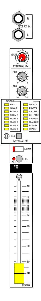
**EXT FX INPUT** TRS jack inputs for connecting the line level stereo output from an external effects processor. The inputs are unbalanced but can also accept balanced sources without modification. The ring connection grounds the -ve (cold) signal to unbalance a connected balanced source.
